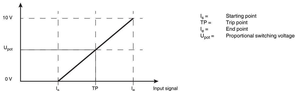
The proportional switching voltage  $U_{pot}$  is calculated using the following formula:
