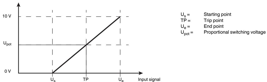
The proportional switching voltage U<sub>pot</sub> is calculated using the following formula:
